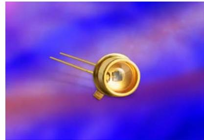
Applications include auto light-dimming (both interior and exterior), fluorescence detection, color sensors, and general daylight detection tasks. Hermetically sealed in a standard TO-46 can, the new selective wavelength device easily integrates into new and/or existing systems. Storage and operating temperatures range from -30 degrees C to 85 degrees C and lead soldering temperature is 260 degrees C.
