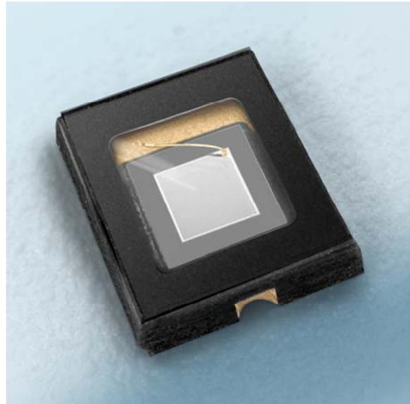
The NXIR-RF100C has an active area of 1 mm<sup>2</sup> in a small 3 mm x 3.5 mm surface-mount package. The new device has high responsivity of 0.62 A/W @ 850 nm and 0.35 A/W @ 1064 nm. It also has low capacitance of 3 pico-farads (pF) at 0 volts, high shunt resistance, greater than 200 MΩ, and very low dark current at 0.1nA. Opto Diode's NXIR-RF100C detectors are available in high volume on tape and reel.
