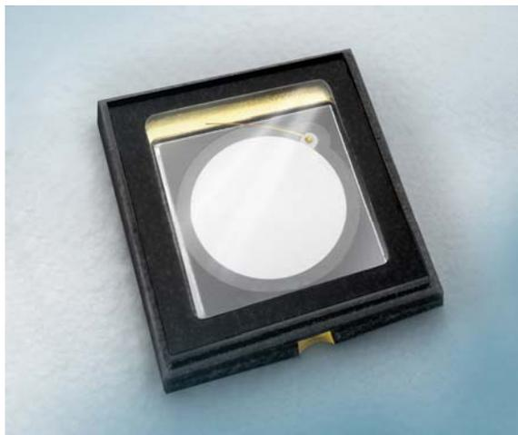
The NIR-enhanced detector is specially designed for laser monitoring, medical diagnostic equipment, industrial automation, scientific measurement, and military applications which require a wide operating temperature range from -40 degrees C to +125 degrees C. The robust package features an AR-coated window that provides greater than 98% transmission. The SMD is compliant with RoHS and REACH standards and is available on tape and reel.
