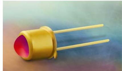
Opto Diode's OD-850L IR LEDs can be stored or operated at temperatures ranging from -40 degrees C to 100 degrees C. The convenient package is ideal for use in optical encoders and photoelectric controls. Peak emission wavelength is 850 nm, the total power output ranges from a minimum 25mW, with a typical output at 35mW, and peak forward current at 300mA. The medium emission angle IR LEDs are available for shipping now at \$2.80 each, minimum order of 100 pieces.
