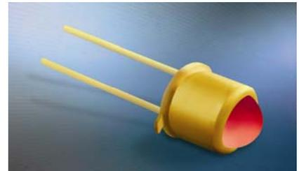
With optical power output of 30mW typical at 100mA and continuous forward current at 100mA, the peak forward current (based on absolute maximum ratings at 25 degrees C) is 300mA. OptoDiode's new OD-850F narrow angle, high power emitter can be stored and operated safely at temperatures ranging from -40 C to 100 degrees C. Shipping now, the new OD-850F devices are economically priced at \$2.80 each, minimum order of 100 pieces.
