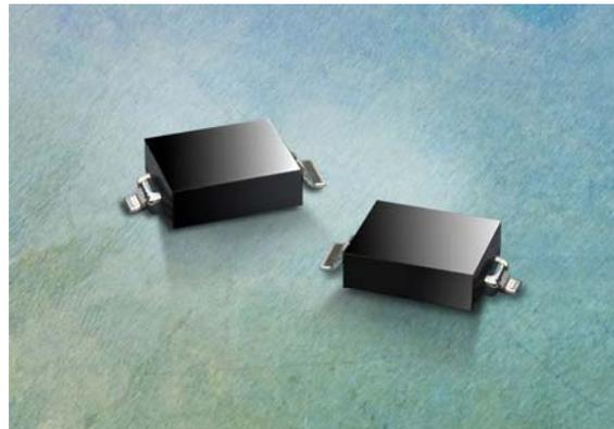
Opto Diode's new ODD-900-001 with daylight filter is highly durable and designed for use in a wide variety of industrial detection tasks. It operates from -25 C degrees to +85 degrees C; the storage temperature range is between -40 degrees C and +85 degrees C. Power dissipation is 150mW at (or below) 25 degrees C (free air temperature). Reliable and rugged, the new device also features a soldering temperature of 260 degrees C (soldering time is 5 seconds, maximum).
