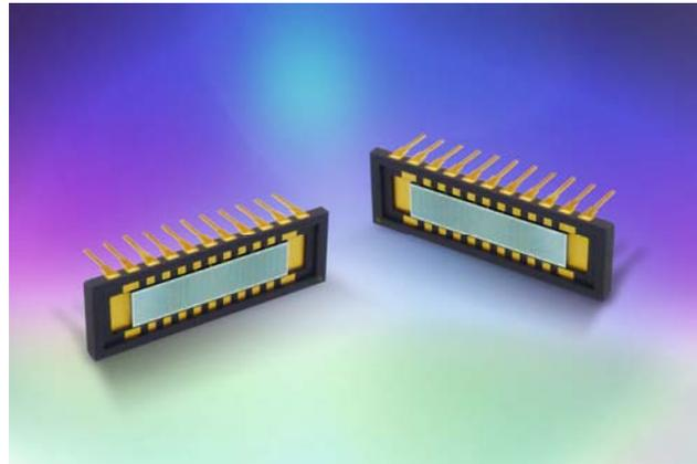
The AXUV20ELG includes an active area of 0.75 mm x 4.1 mm and a sensitive area of 3 mm<sup>2</sup> per element. The reverse breakdown voltage is typically 25 volts and the capacitance is 40 pF maximum (at 25°C, per element). With a rise time of 200 nsec and shunt resistance (per element) at a minimum 100 MOhms, Opto Diode's new 20-element photodiode provides exceptionally stable response after exposure to high energy radiation.
