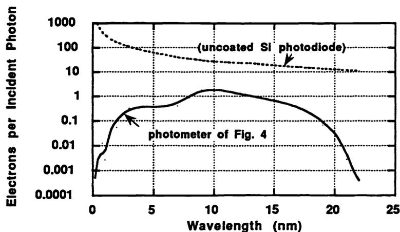
Figure 5. The calculated efficiency of a single-reflection photometer of the type shown in Fig 4. The spectral bandpass can be modified by choices of reflector material, grazing angle, and filter material. The calculated efficiency of an uncoated silicon photodiode alone is also shown.
