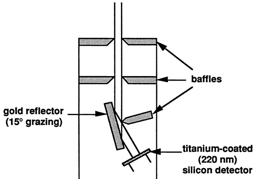
Figure 4. Example of a single reflection photometer design configured to reduce response to x-rays.
