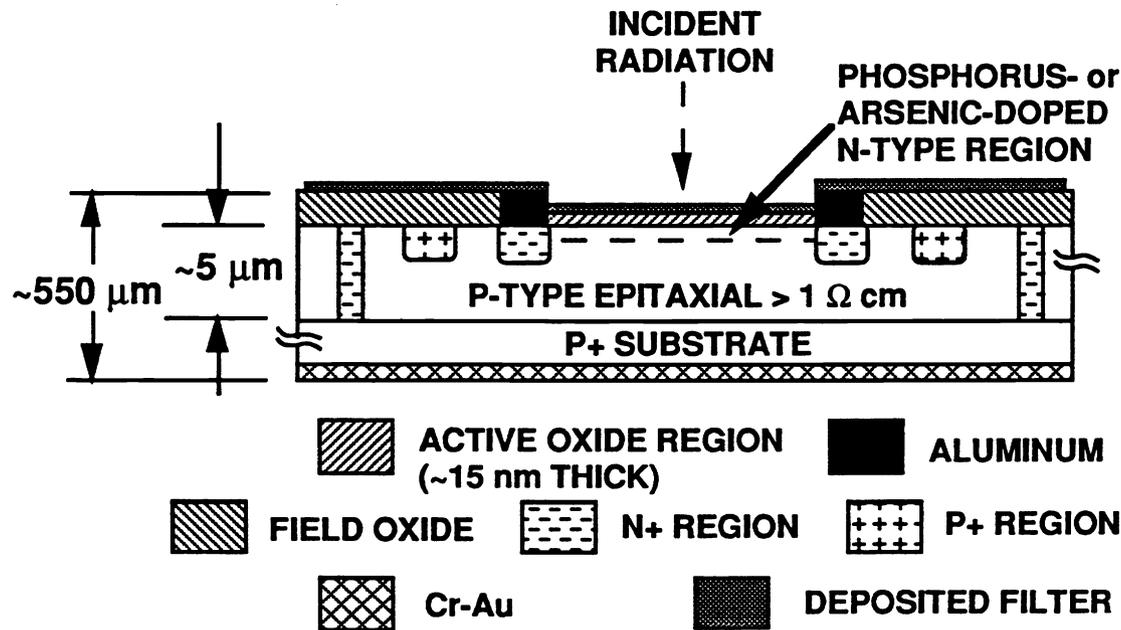
Figure 1. Schematic of the optically filtered EUV photodiodes prepared for this study.
