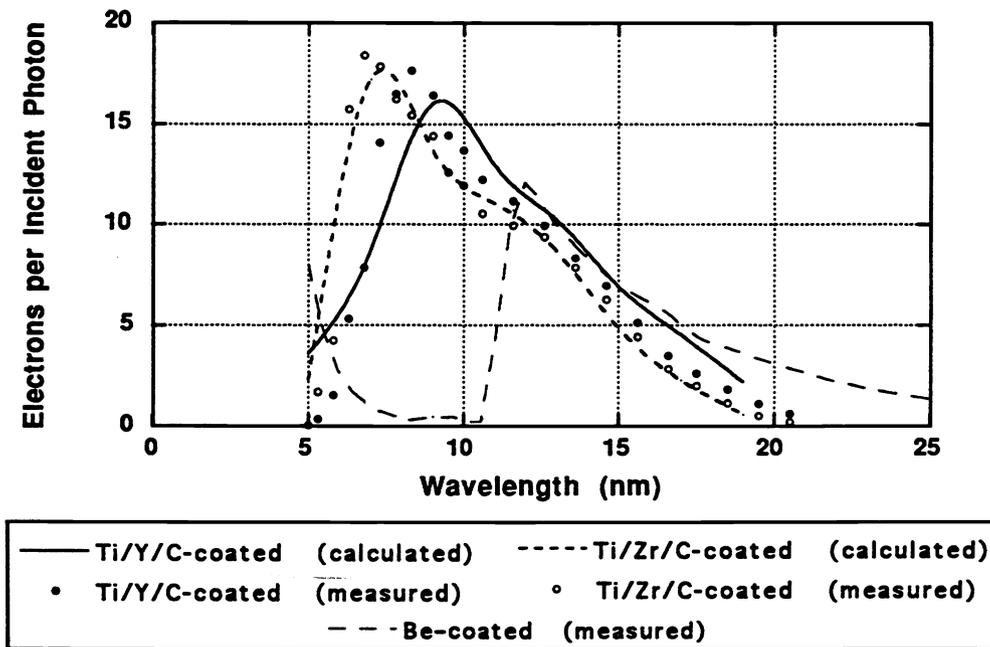
**Figure 3** The measured and calculated response of silicon photodiodes coated with Ti/Y/C (6 nm/210 nm/55 nm) or Ti/Zr/C (6 nm/195 nm/50 nm) with the response of a photodiode coated with Be (400 nm) shown for comparison.
