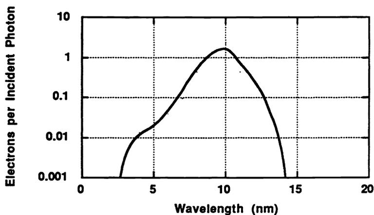
Figure 6. The calculated efficiency of a single reflection photometer utilizing a silver mirror and a silver coating on the surface of a photodiode. The calculations do not include surface films.
