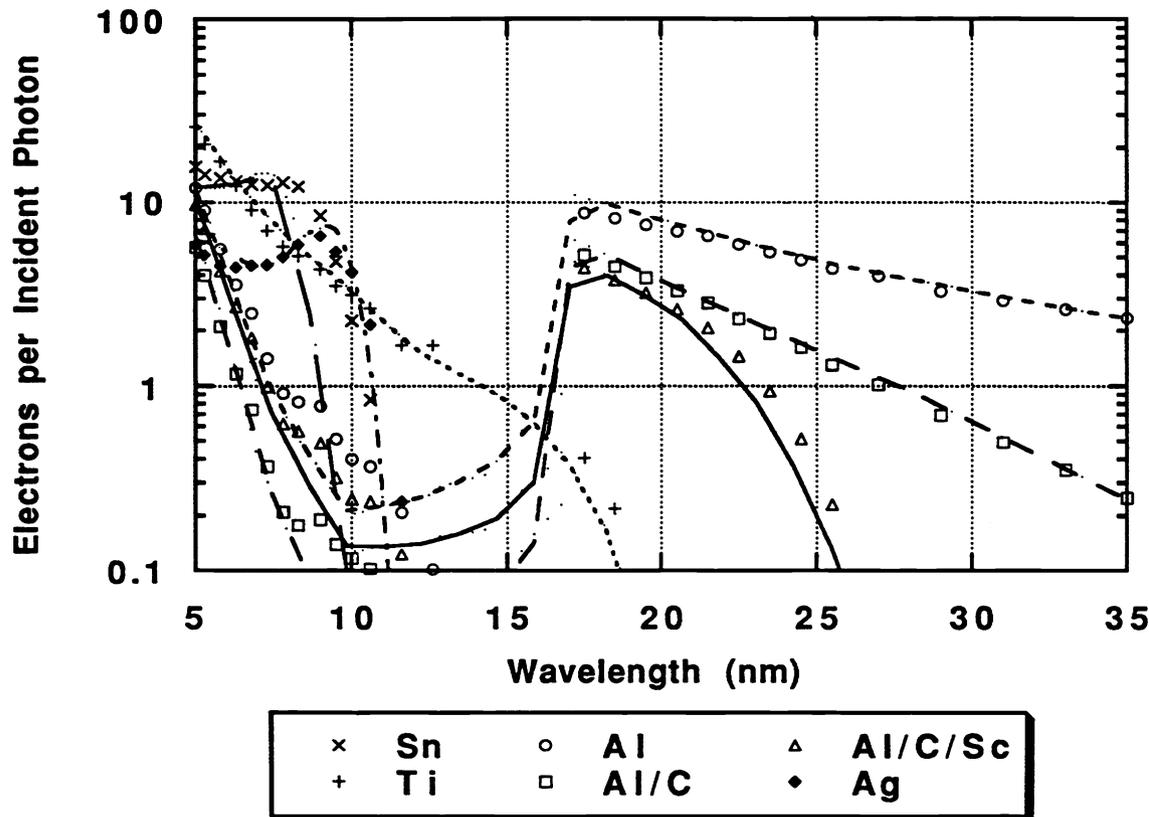
Figure 2. Calculated (curves) and measured (points) efficiencies of silicon photodiodes coated with several common EUV filtering materials. Calculations included losses in the filters, and in the SiO<sub>2</sub> passivating oxide on the photodiode surfaces. The effective film thicknesses used in the calculations are given in Table 1.
