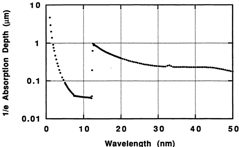
Figure 7. Calculated 1/e absorption depth in silicon as a function of wavelength.
