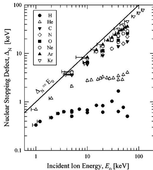
FIG. 2. Nuclear stopping defect  $\Delta_N$  for silicon detectors, which is shown as a function of incident ion energy, is due to the interaction physics of an ion in the detector material and fundamentally limits the output pulse magnitude from SSDs.
