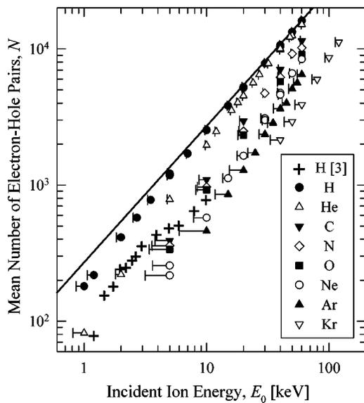
FIG. 1. Measured number of electron-hole pairs is shown as a function of the incident energy for several ion species and represents the maximum pulse magnitude possible from a silicon SSD. The line represents the case in which all of an ion's energy is lost to processes that generate electron-hole pairs. The  $H^+$  data shown as (+) are from a back-thinned delta-doped CCD (Ref. 3).
