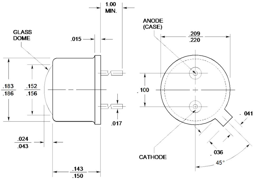
All surfaces are gold plated. Dimensions are nominal values in inches unless otherwise specified. Window caps are welded to the case.
