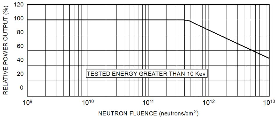
Typical Degradation Curve
