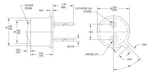
All surfaces are gold plated. Dimensions are nominal values in inches unless otherwise specified. Caps are welded to the case.
