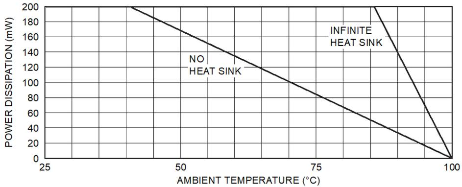
Typical Degradation Curve
