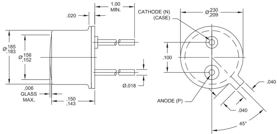
All surfaces are gold plated. Dimensions are nominal values in inches unless otherwise specified. Window caps are welded to the case.
